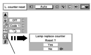
Move pointer to Lamp counter reset and then press SELECT button. Message "Lamp replace counter reset?" is displayed.
